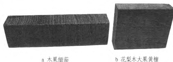
图 3 木果缅茄木(左)与花梨木大果紫檀(右)木材试样外观 Fig. 3 Appearance comparison between Afzelia xylocarpa and Pterocarpus macarocarpus wood samples
